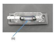
Use a TORX T20 screw drive to open two screws. Rear plate lamp and be remove and replaced by hand as shown in (6) Note: the lamp is C5W
