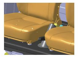
Hand brake rod is located between the two seats shown Hand brake applies brake on the front wheels.
